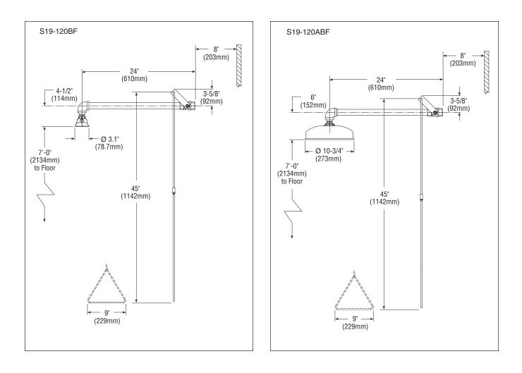
NOTE: All dimensions assume standard thread engagement. Variations in manufacturing allow for +/- 1/8" (3mm) per threaded joint. To find the tolerance of a dimension, add the number of thread joints in between a dimension and multiply it by 1/8" (3mm).
